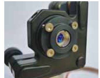
Mounted PCA with aspheric focusing optical lens
