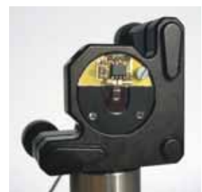
Detector antenna with preamplifier
