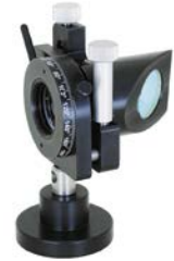
Variable Attenuators for linearly polarized laser beam 990-0071 page 5.12
