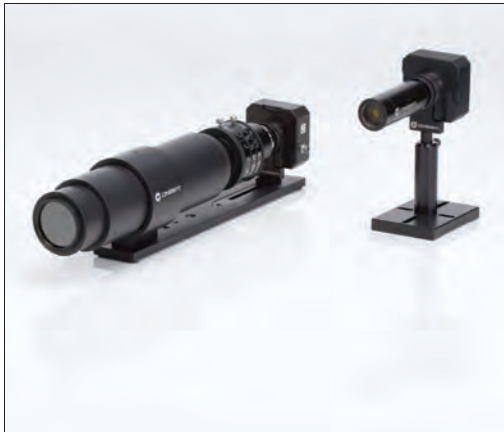
BIP-5000Z and BIP-12F attached to a LaserCam-HR
