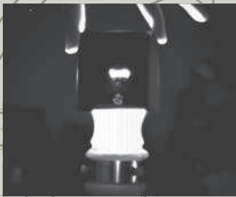
IR filter testing – looking through glass
